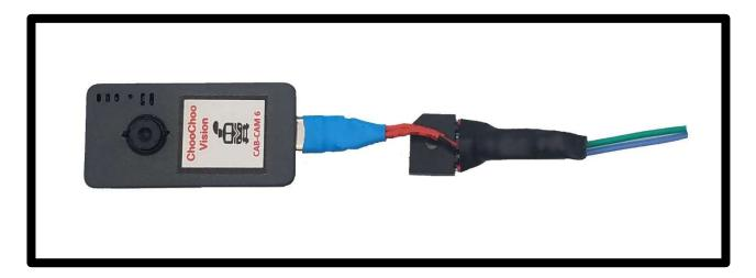
**Battery**: Your CCV Camera contains an internal battery. The battery is designed to be used as a keepalive in concert with a DCC Power converter. The battery is automatically recharged from track power using the DCC Power Converter.
